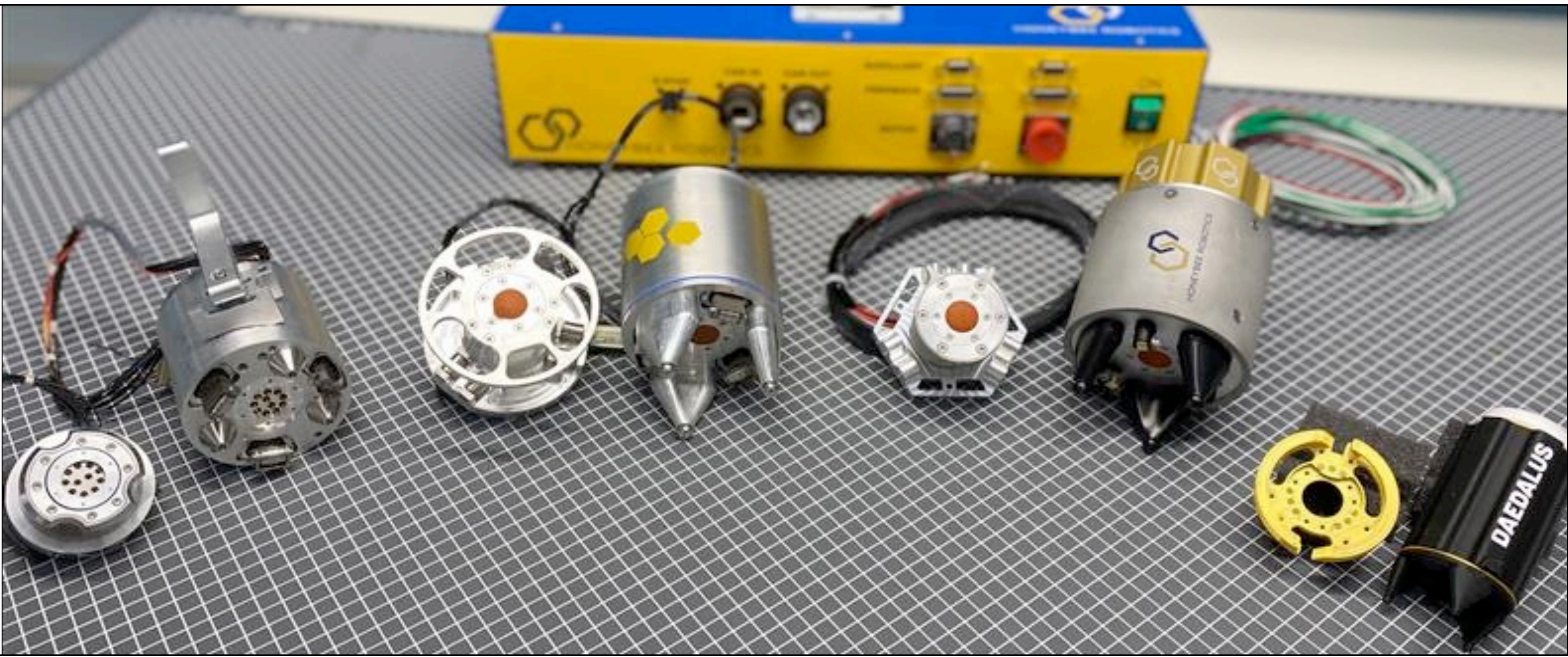
Figure 1. Honeybee Robotics Dust Tolerant Electrical Connector Lineage; Left to Right: c. 2011 Socket Unit & Manual Plug, c.2012 Socket and Motorized Plug, c.2023 Socket & Manual Plug, c.2024 A 3D Printed Prototype Of The Latest Socket and Manual Link Units
