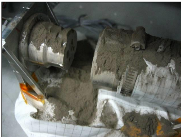
Figure 1. TRL 6 DTC undergoing dirty TVAC testing
